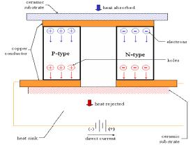
Fig: 2. Current Flow in P-N Junction
