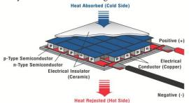
Fig: 5. A Cutaway of Thermoelectric Module
